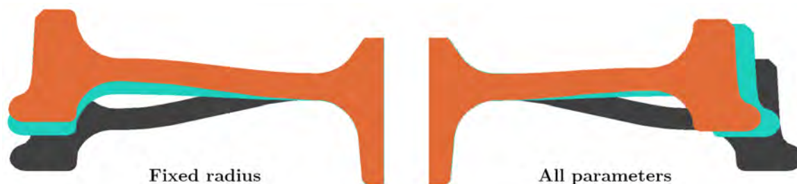
Figure 4: Wheel shapes comparison for the BFSs obtained by the optimization procedure with the fixed radius case (left) and considering all the geometric parameters (right). In both cases the results are shown for the NF-max (orange) and L_{A,W} -min (green) approaches together with the reference wheel (black).
