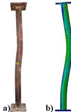
Fig. 10. Experimental (a) and numerical (b) configurations of a deformed CHS column after test.
