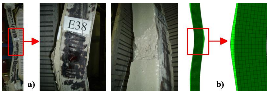
Fig. 9. Experimental (a) and numerical (b) configurations of a deformed composite H column after test.
