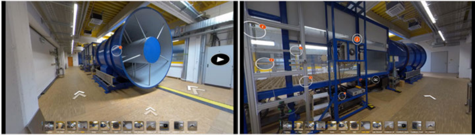
Figure 1. 3D virtual representation of the Boundary Layer Wind Tunnel at the Ruhr-Universität Bochum - remote access points are marked "i" and show explanations about steering and sensing of experiments as well as videos of specific experiments; experimental parameters can be varied within a certain range, corresponding data from previous experimental campaigns can be downloaded for further processing.
